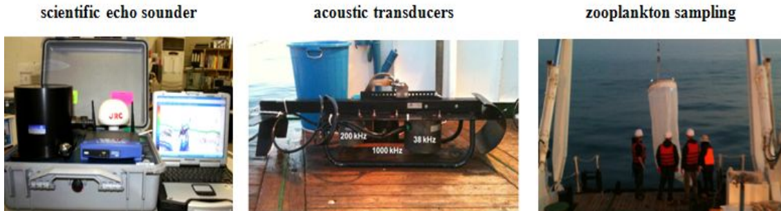
Fig. 3.6.1.2 Experimental set up for hydroacoustic surveys.
