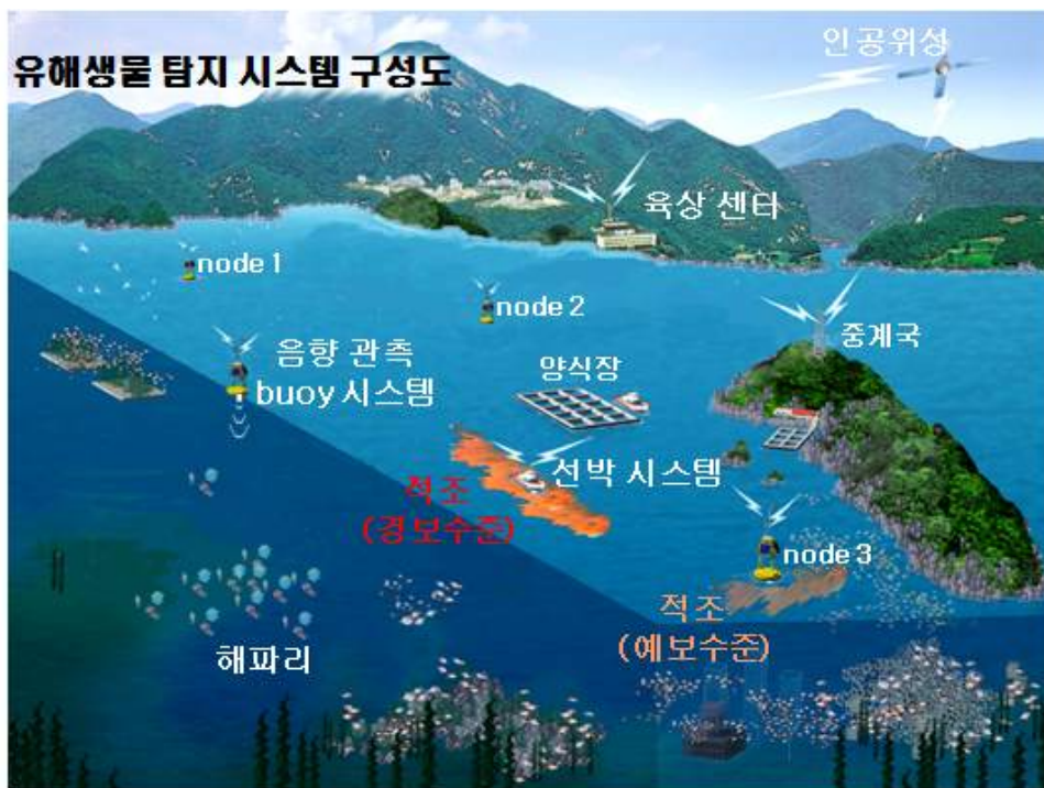
Fig. 10. System schematic of real-time red tide detection using acoustic system.
