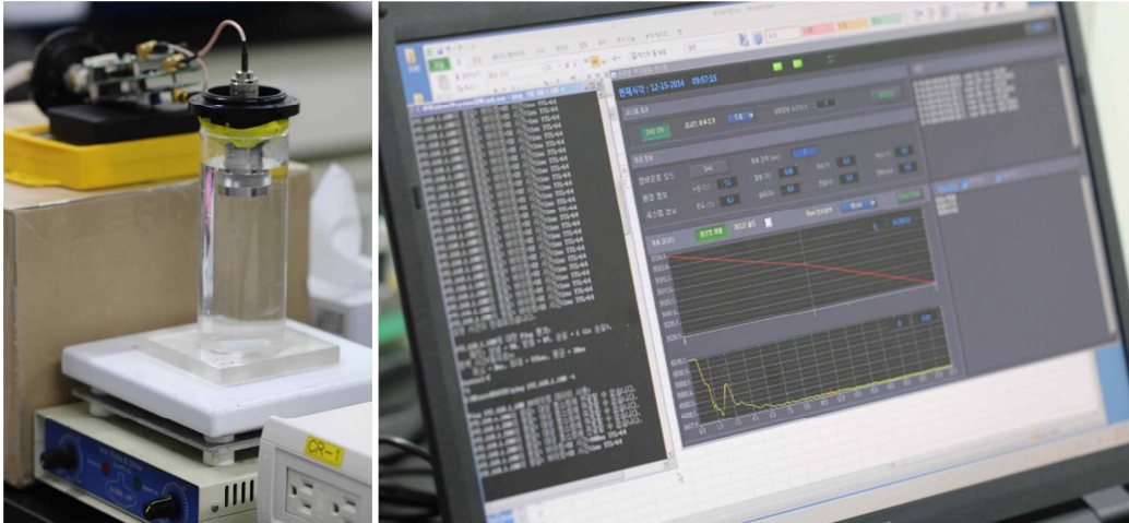
Fig. 23. Photographs of analysis of each cell concentration of HABs and natural phytoplankton community in 1 L culture flask using the acoustic system for real-time detection of the harmful algal blooms.
