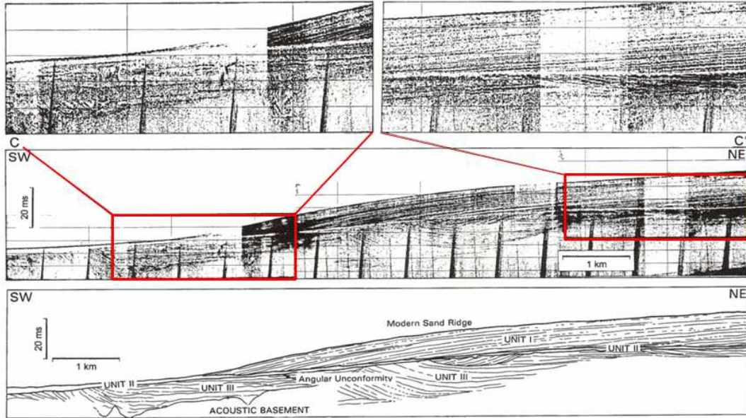
Fig. 7.—High-resolution seismic section (C-C') from the middle part of nearshore sand-ridge zone (for location, see Figure 4) and its interpretation. Unit I comprises a seaward-migrating sand ridge with downlapping internal reflectors, whereas Unit II is acoustically transparent and thin, consistently draping the somewhat flat surface of Unit III. Within Unit III, an angular unconformity at the top and locally deformed reflections can be seen.
