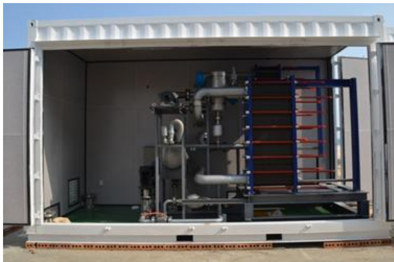
<A photo of 20 kW OTEC plant>
