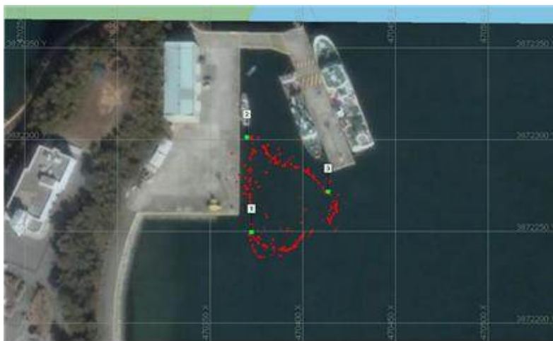
Fig. 6.2.1 Tracking results in Hypack monitoring program
