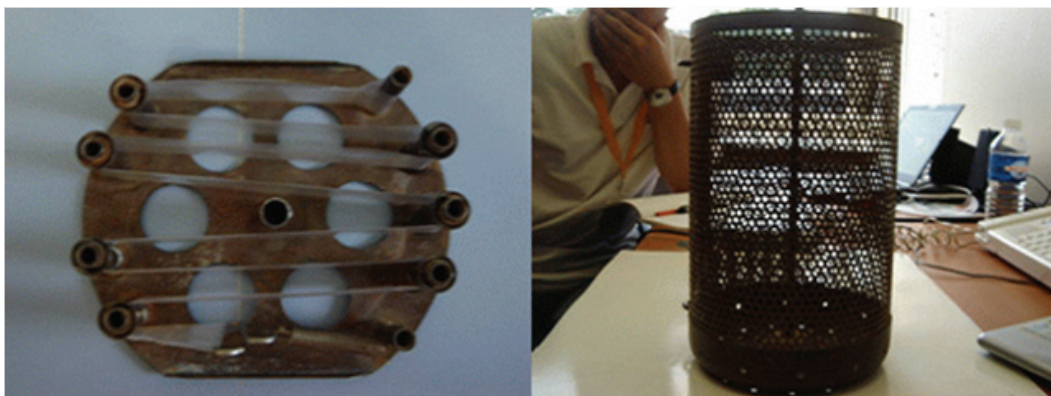
Fig. 3-4-6. SPMD and LDPE-type passive sampler.
