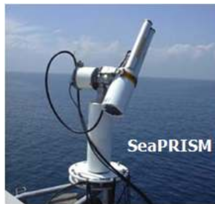
Figure 2.3 SeaWiFS Photometer Revision for Incident Surface Measurements (SeaPRISM) of the Aerosol Robotic Network (AERONET)
