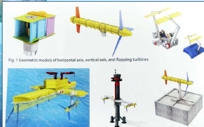
Fig. 2 Horizontal axis turbine combined with floating, pile, and gravity type sub-structures
