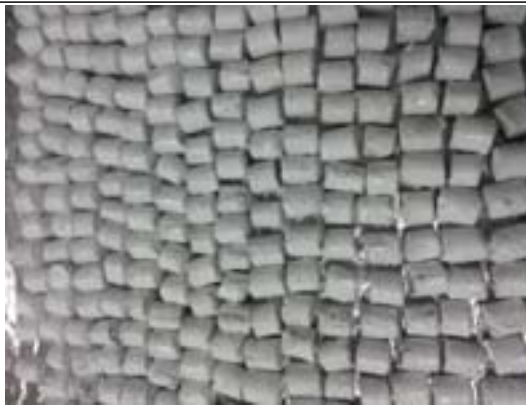
Polysulfone coating(double coating-mixing of polysulfone and N,N-dimetyl acetamide)
