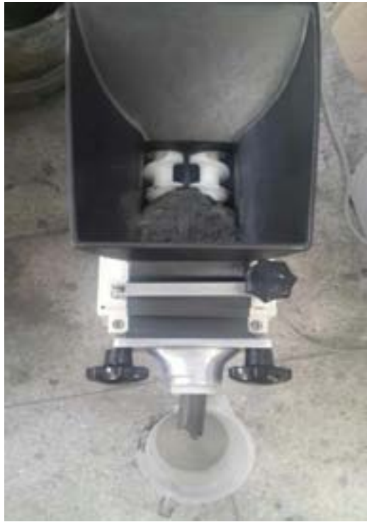
Making pellets and biostimulant balls dried at 60°C for 48hr
