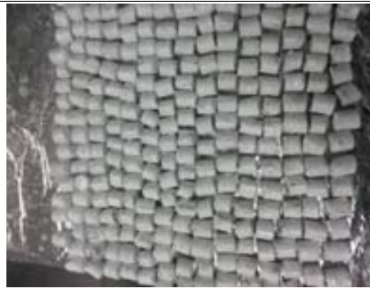
Polysulfone coating(double coating-mixing of polysulfone and N,N-dimetyl acetamide)
