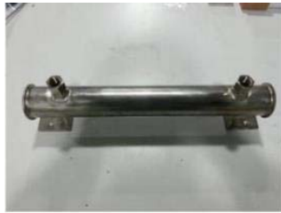
In/Out: 15A(PT 1/2") Shell: 50A SUS pipe, SCH10S, 길이 470mm Tube: Ø12mm, t1mm, SUS316
