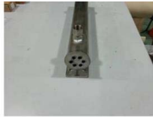
In/Out: 15A(PT 1/2") Shell: 50A SUS pipe, SCH10S, 길이 470mm Tube: Ø12mm, t1mm, SUS316
