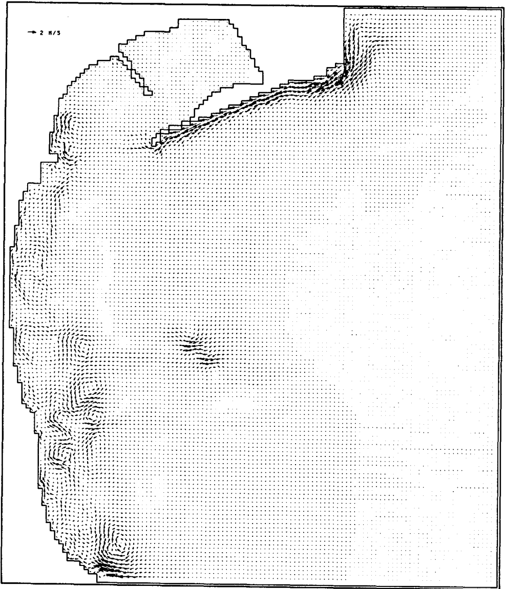
Fig. 3.3.9. Computed wave-induced current vectors for the present state (wave direction of ENE).
