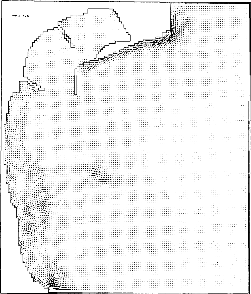
Fig. 3.3.10. Computed wave-induced current vectors for the KMPA plan (wave direction of ENE).
