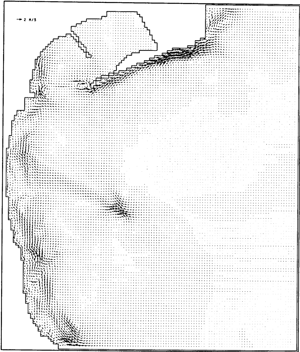
Fig. 3.3.15. Computed wave-induced current vectors for the present state (wave direction of ESE).
