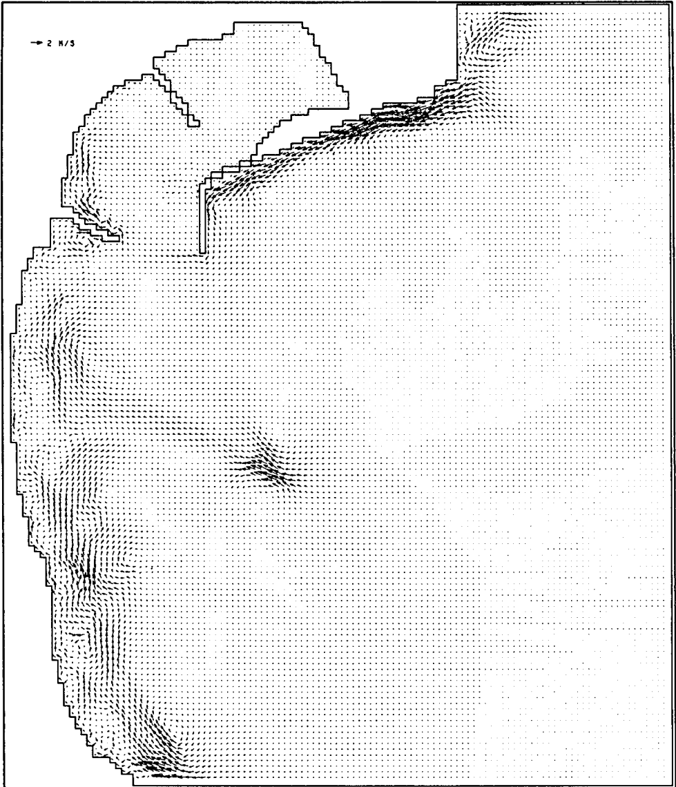
Fig. 3.3.16. Computed wave-induced current vectors for the KMPA plan (wave direction of ESE).
