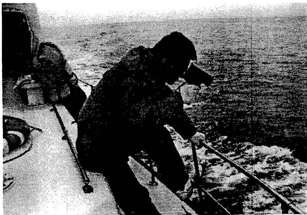
Fig. 2-6. In-situ measuring of SST using Minolta SPOT DP-210 infrared thermometer.
