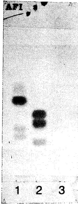
Fig. 3-6-4. TLC analysis of sugars from whole hydrolysate of strain AF-1.
