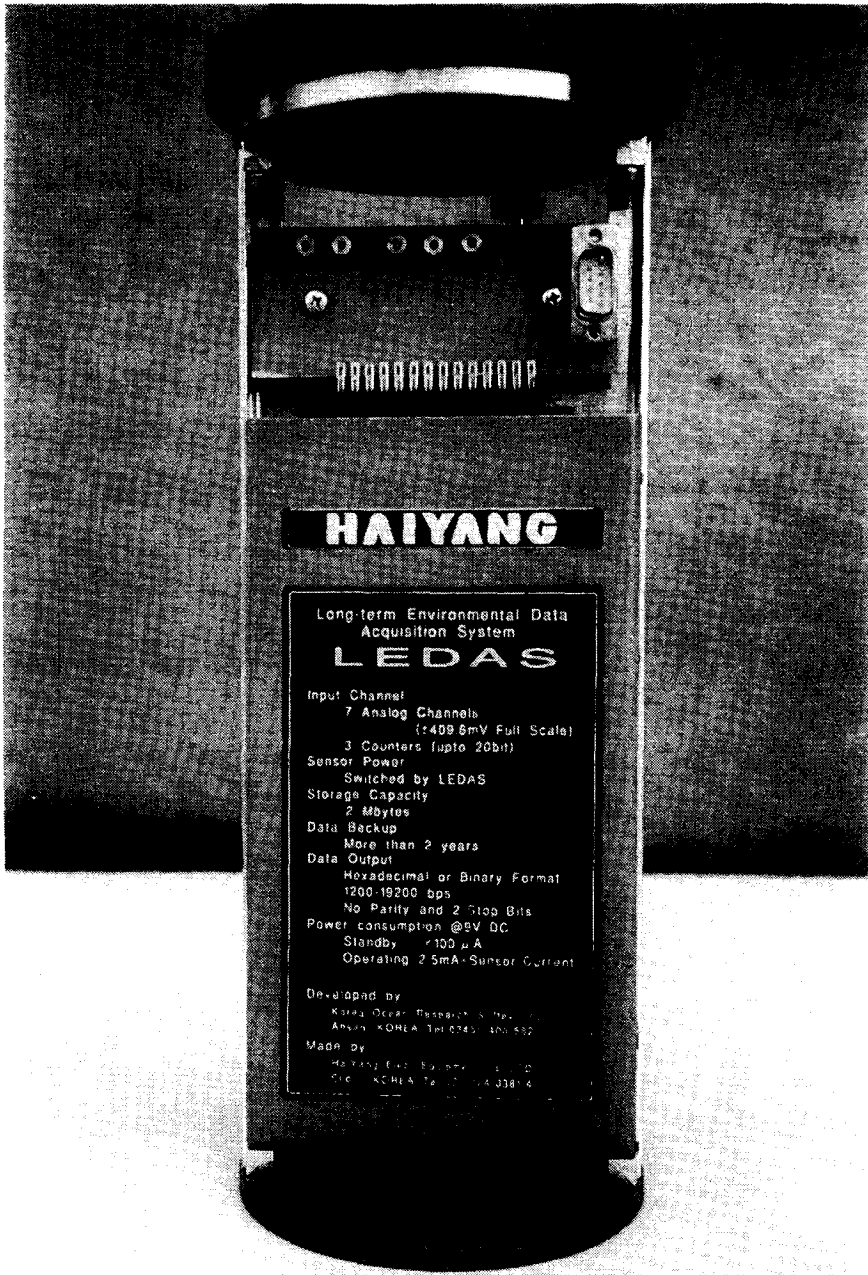
Fig. 6 LEDAS installed in the inside frame of wave gage
