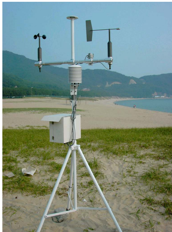
Fig. 5.3. The wireless automatic weather system.
