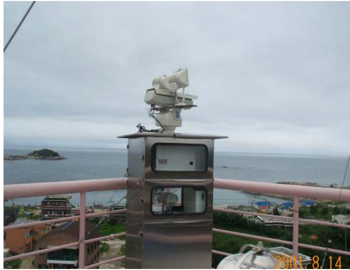
Fig. 5.1. It is take a picture of the installation of visibility monitoring system.
