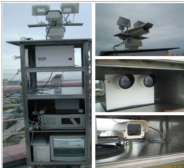
Fig. 5.2. Visibility monitoring system and the part of this equipment.
