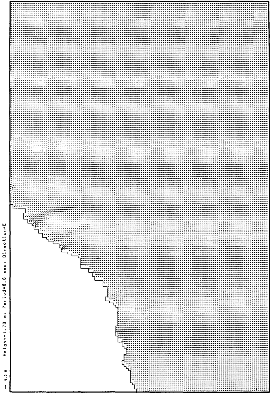
Fig. C.1.7 Calculated wave direction vectors using 10 % annual occurrence wave condition(Dir = E).
