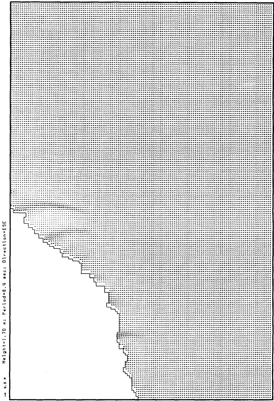
Fig. C.1.2 Calculated wave direction vectors using 5 % annual occurrence wave condition(Dir = ESE).
