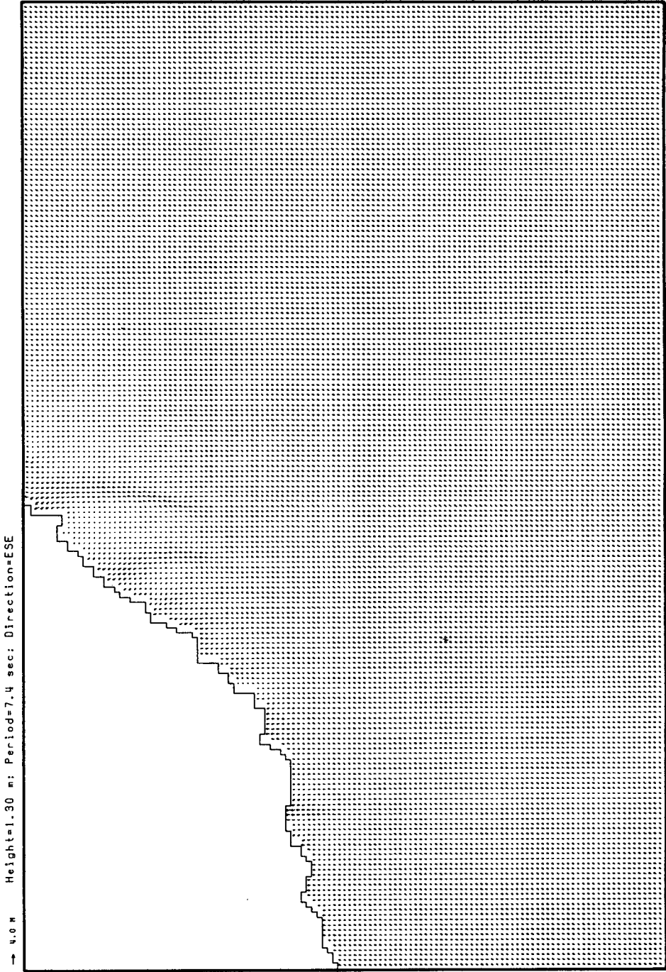
Fig. C.1.6 Calculated wave direction vectors using 10 % annual occurrence wave condition(Dir = ESE).
