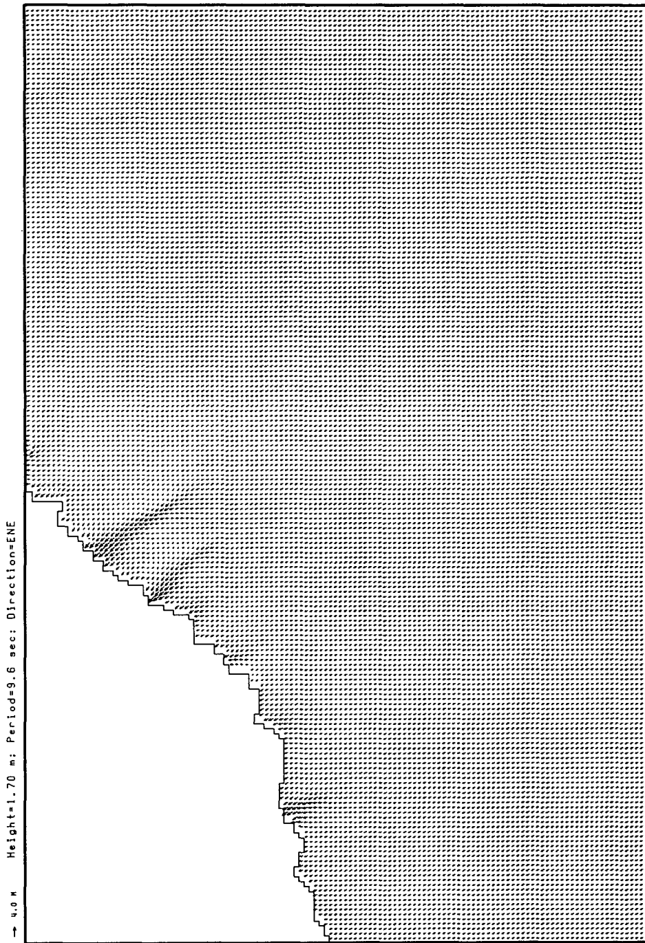
Fig. C.1.8 Calculated wave direction vectors using 10 % annual occurrence wave condition(Dir = ENE).
