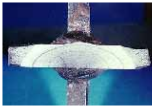
Development of fatigue crack growth in welded specimen. Beachmarks produced by block loading.
