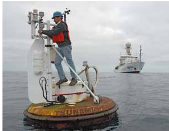
Staying On Top of His Work. Senior engineering assistant Jeff Lord of the WHOI Upper Ocean Processes Group adjusts and services the instruments atop a deep-ocean moored buoy on October 27, 2007. The research vessel Ronald H. Brown looms in the distance. Working off the Pacific coast of Chile, the research team has been examining the exchange of heat, moisture, and momentum between the ocean and atmosphere, while also providing data for tsunami detection. (Photo by Sean P. Whelan, Woods Hole Oceanographic Institution)
