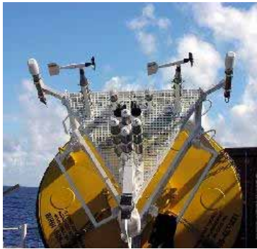
The ASIMET system consists of seven modular sensors that can be mounted on ocean buoys or ships. For calibration and backup during long studies, scientists often deploy two full sets of sensors at a time. (photo courtesy Robert Weller)
