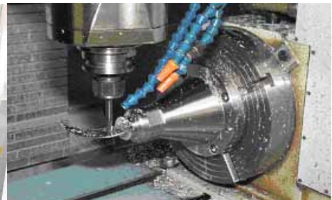
milling of a propeller model in bronze. Before leaving the milling machine, each blade has been through a control measurements.
