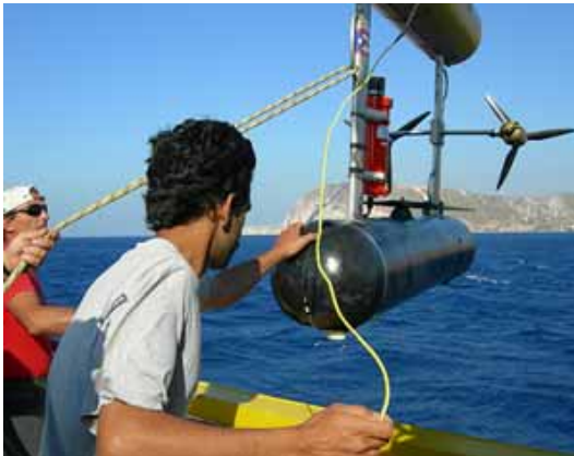
Off It Goes! WHOI engineer Hanumant Singh (center) helps deploy the autonomous underwater vehicle (AUV) SeaBED in the Aegean Sea during recent archaeological studies. Singh took part in the Project PHAEDRA 2006 expedition to explore an ancient shipwreck. (Photo by Matthew Barton, Woods Hole Oceanographic Institution)
