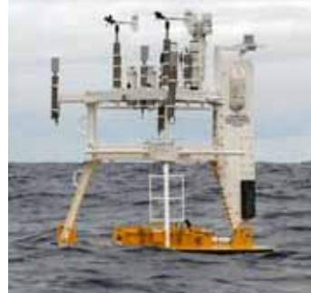
A buoy ready for recovery at the STRATUS site off Chile in the Pacific Ocean. The aluminum buoy is riding low in the water after a year at sea - one good reason why Surlyn foam buoys, which don't leak, are now routinely used.
