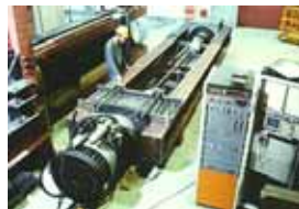
Fatigue testing of 75 mm diameter steel rope.
