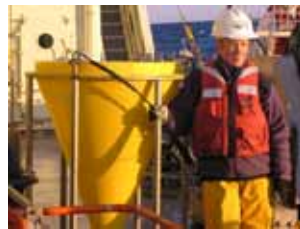
Sediment traps are some of the biggest instruments used in ocean moorings. The funnel openings are made large to catch enough sediment for analyses. Here, Cynthia Pilska, of Bigelow Laboratory for Ocean Sciences, heads out on R/V Oceanus to deploy a trap. (Patrick Rowe, WHOI)
