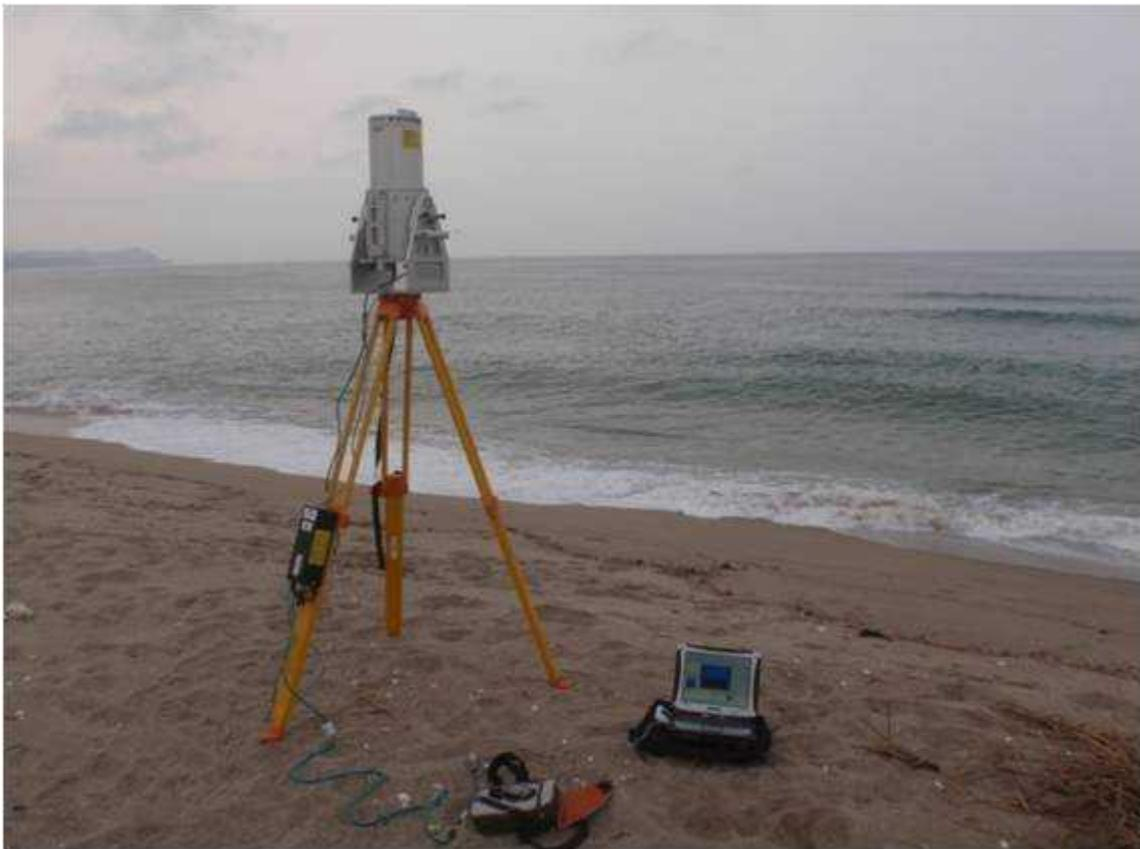
Figure 3. Terrestrial LiDAR system used in this study.
