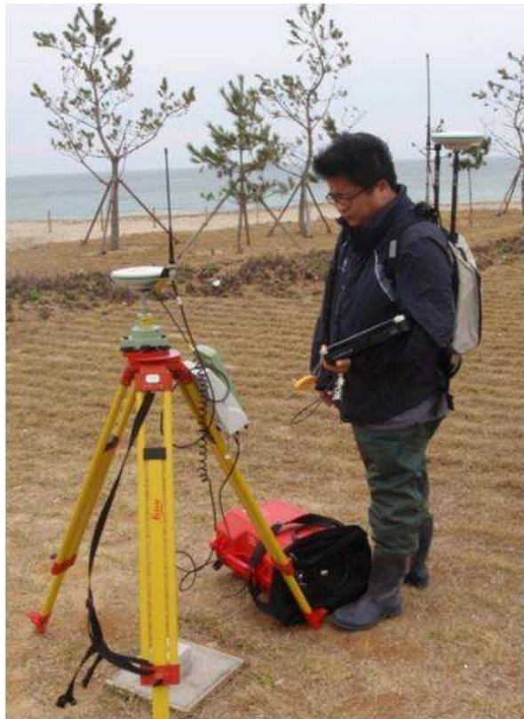
Figure 4. Beach topography surveying system using the RTK-GPS system
