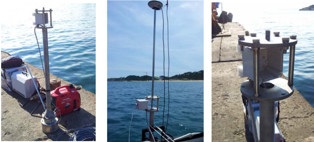
(a) Frame of echosounder (b) Frame of antenna (c) Box of motion sensor
