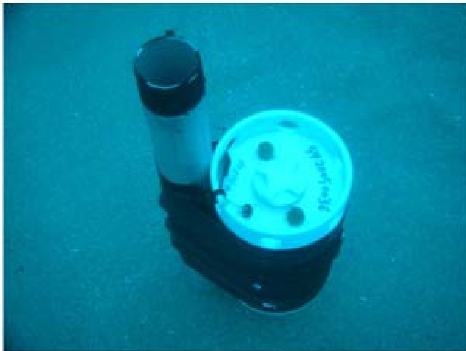
Fig. 3. 2. 2. 2. Pressure type wave/tide gauge installed at the test site
