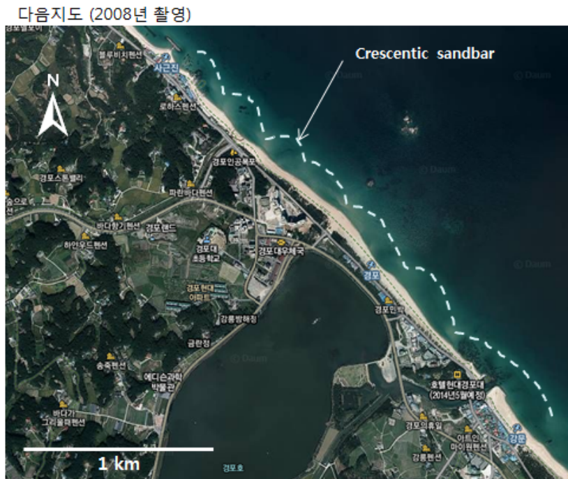
Fig. 3. 3. 3. 1. Example of crescentic sandbar in airborne photography
