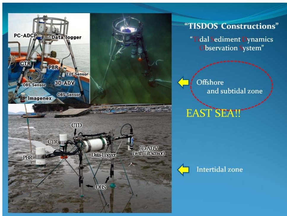
Fig. 3. 3. 2. 1. TISDOS (Tidal Sediment Dynamic Observational System)
