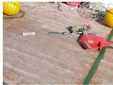
그림 1. Photographs of the self-recording hydrophone attached to the mooring line.
