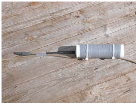
그림 1. Photographs of the self-recording hydrophone attached to the mooring line.
