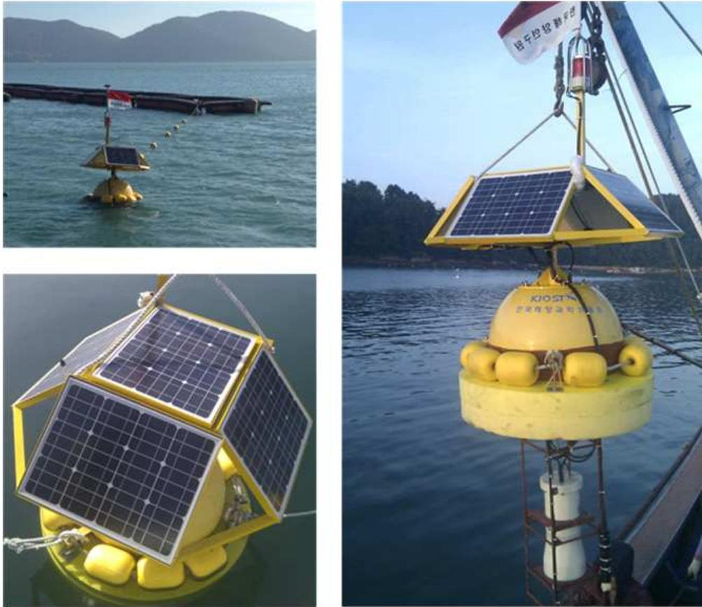
Fig. 3.2.104. Photography of acoustic detection system from buoy-type.
