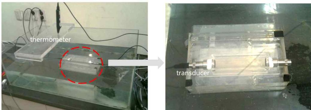
Fig. 3.2.41. Experimental set up for sound speed of red tide.
