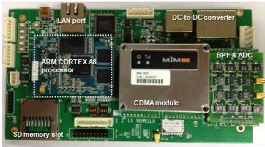
Fig. 3.2.91. Signal analysis/system control board.
