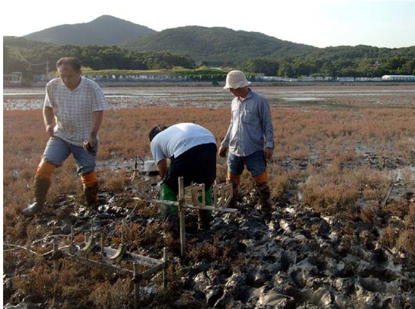
Fig. 3-1-11. Artificial disturbance of the VMF bed during instruments installation.
