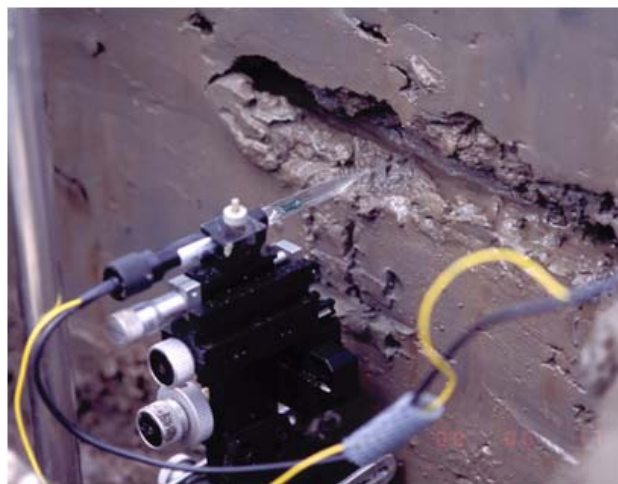
Fig. 3-2-115. Horizontal oxygen measurement from burrow walls with an oxygen micro-electrode and a manuplator.
