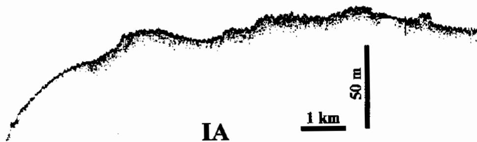
Fig. 6-41. Part of seismic profile showing typical feature of the Echo facies IA.
