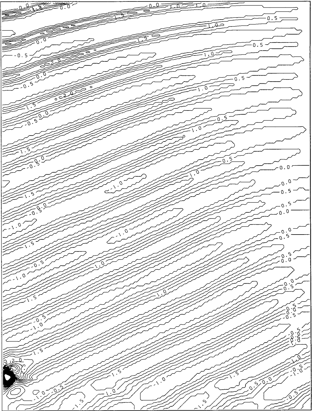
Fig. 2.4.10 Contour of water surface elevations at t = 500 seconds and P8(regular waves 30^\circ obliquely incident to J- axis).
