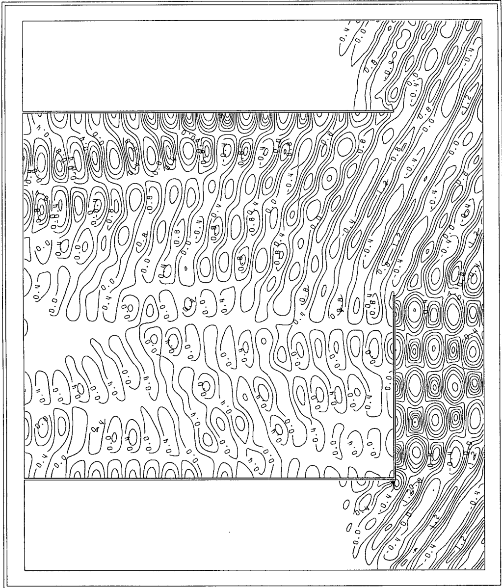
Fig. 2.4.19 Contour of water surface elevations around the harbor at t = 600 seconds (regular waves -30^\circ obliquely incident to J-axis).
