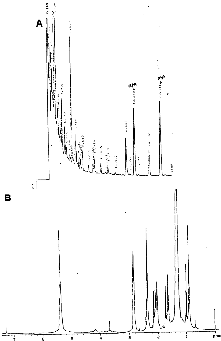
Fig. 5.8. GC chromatogram of total Fatty acid of hydroid Solanderia secunda (A), producing Eicosapentaenoic acid (EPA, C20:5), and Docosahexaenoic acid (DHA, C22:6), and NMR spectrum (B).
