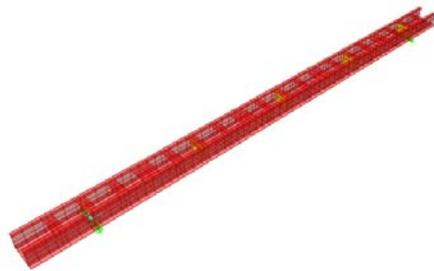
Figure 9. Numerical analysis model (SAP2000)
