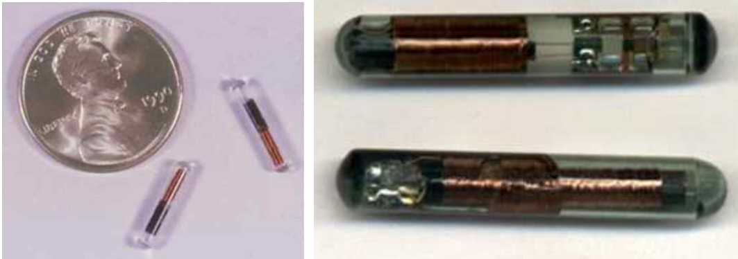
그림 2-3-15. PIT tag. (출처: Atlantic States Marine Fisheries Commission: http://www.fishtag.info/index.htm )
