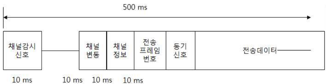
Fig. 60. Transmission frame structure of adaptive AUV acoustic communication modem
