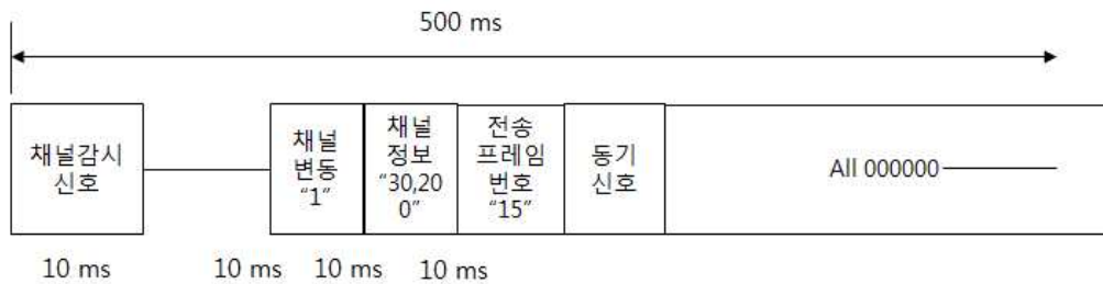
Fig. 61. Transmission frame structure of adaptive AUV acoustic communication modem
