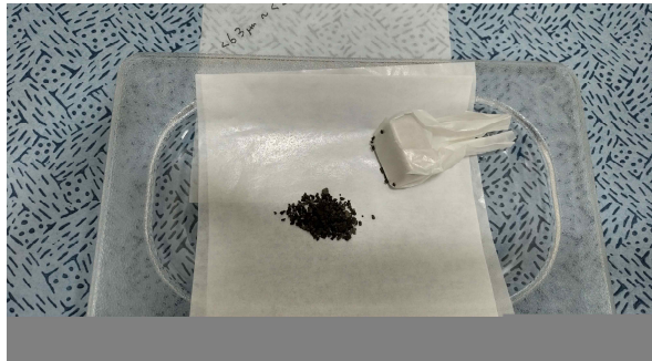
Figure 3.2.4.34. Magnetic separation of MSP from manganese nodule particles by a permanent magnet
