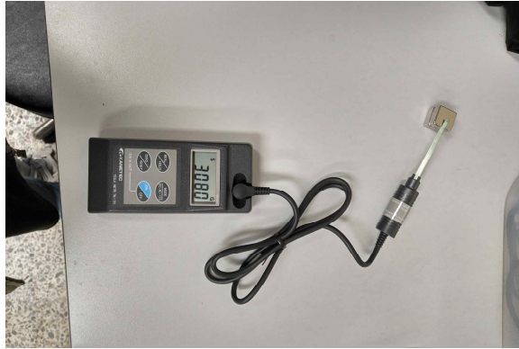
Figure 3.2.4.33. The permanent magnet used for the separation of manganese nodule particles and measuring the strength of the magnet
