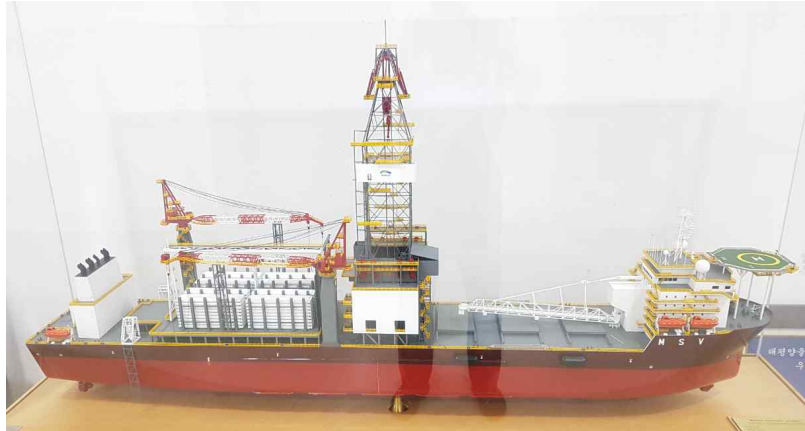
Figure 3.2.4.40. Conceptual model of deep-sea mining vessel (Length 265.1 m, Width 42 m)
