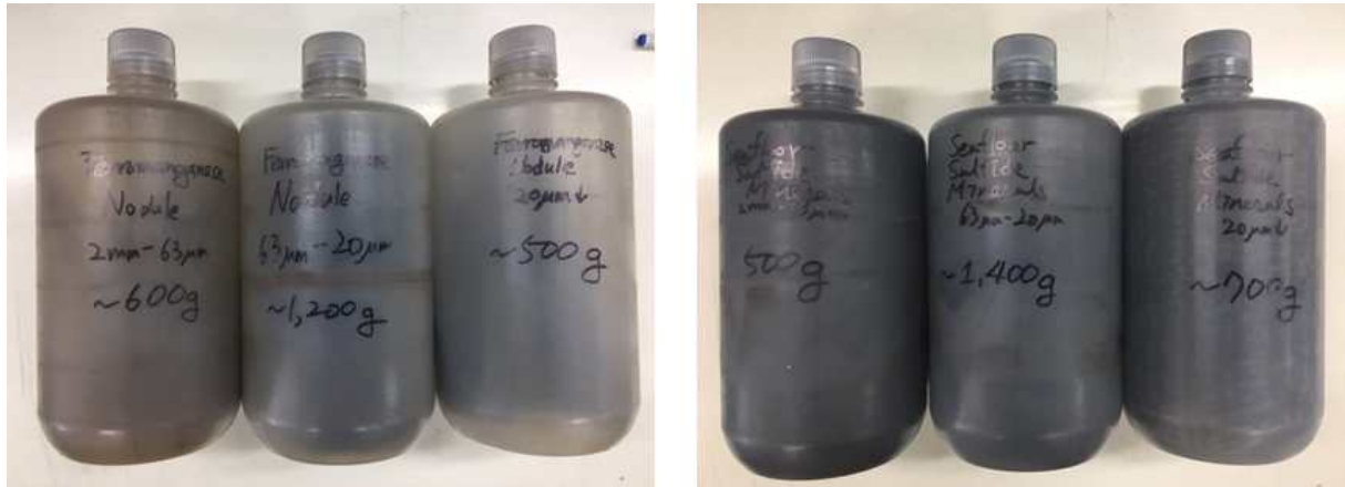
Figure 3.2.1.1. Standard samples for leaching and toxicity experiments by different size of manganese nodule and sulfide minerals
