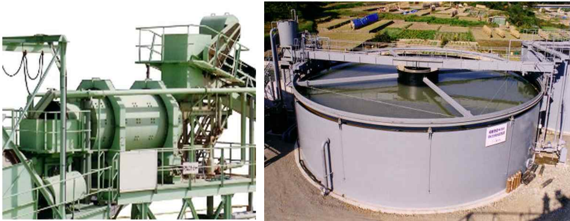
Figure 3.2.4.1. Commercial remediation treatment plant (Ex.: particle separation(left), wastewater treatment(right))
