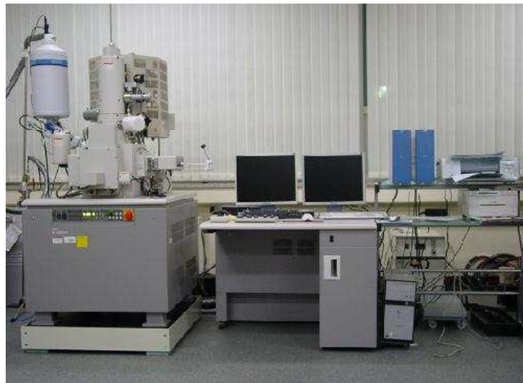
Figure 3.2.4.35. Field Emission Scanning Electron Microscope (FE-SEM), (S4800, HITACHI)
