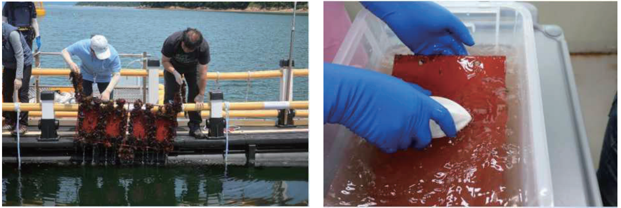
Fig. 3.1.2.16. Retrieving plates placed for 2 months in the seawater (left) and simulated in-water cleaning using brush to remove biofouling on the plates (right).
