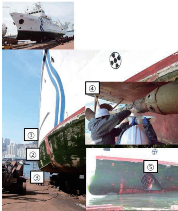
Fig. 3.3.1.23. Sampling of fouling macrozoobenthos at starboard and propeller on the R/V EARDO.
