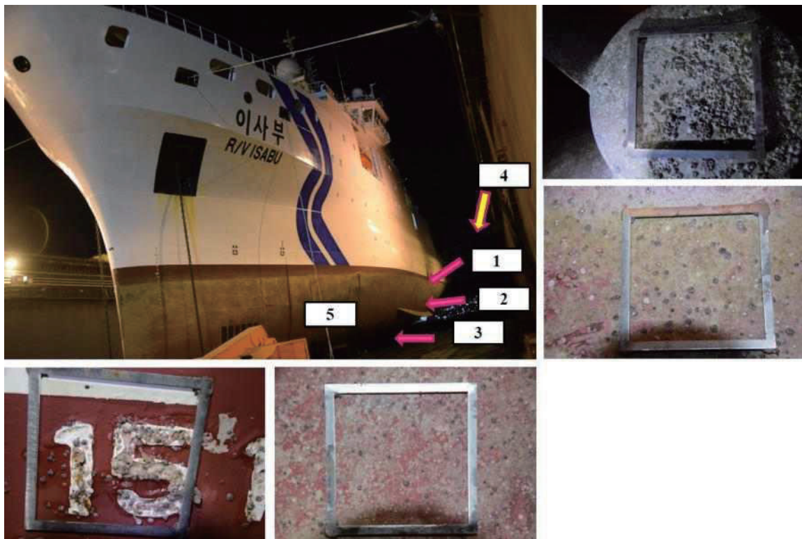
Fig. 3.3.1.26. Sampling of fouling macrozoobenthos at starboard and propeller on the R/V ISABU.
