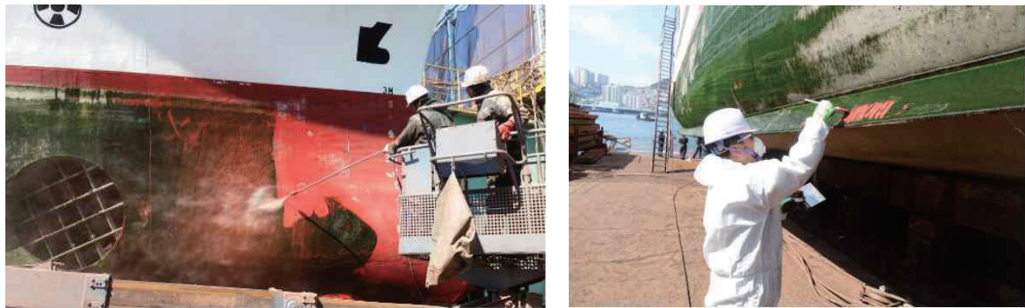
Fig. 3.1.2.1. Hull cleaning with jet water spraying (left) and by scrapping (right).
