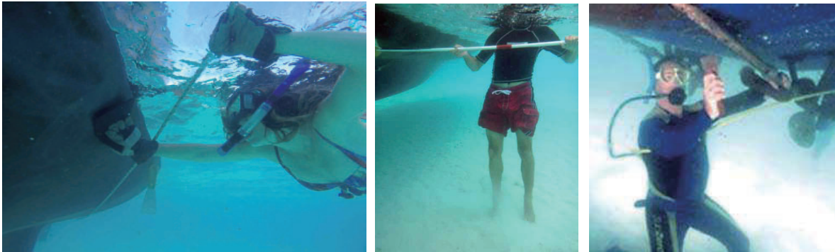
Fig. 3.4.1.1. Photographs of manual brushing (left and middle) and scrubbing (right) by diver.
