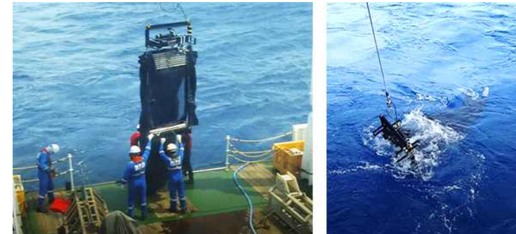
Fig. 3.5.2.3. Multiple Opening and Closing Net Environmental Sensing System (MOCNESS) attached to R/V ISABU
