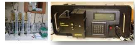
Fig. 3.5.2.6. Analysis of chlorophyll-a using fluorometer (Turner-Designs 10-AU)
