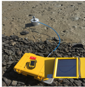
Fig. 7. CH 4 and CO 2 diffuse fluxmeter and a handheld computer (PDA) that allows geo-referencing of acquired data.
