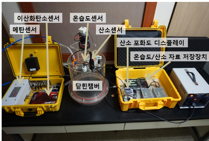
Fig. 2. A closed flux chamber equipped with detectors for CH 4 , CO 2 , O 2 , air temperature, and humidity.
