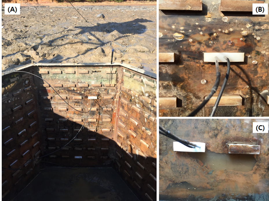
Fig. 6. A hexagonal acrylic observatory for in situ oxygen content in the burrow (A) and silicone-filled holes in the acrylic walls allowed direct measurement in intact burrows with optode oxygen sensor (B, 30 cm depth and C, 90 cm depth).
